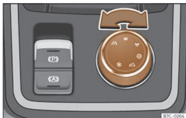
Fig. 141 Console centrale : Commande rotative (Driving Experience button).
