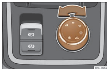
Fig. 143 Console centrale : Commande rotative (Driving Experience button).
