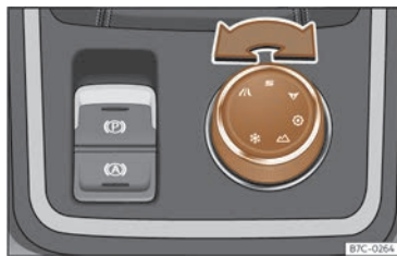
Fig. 96 Console centrale : Commande rotative (Driving Experience button).
