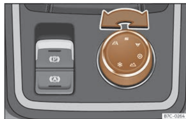
Fig. 95 Console centrale : Commande rotative (Driving Experience button).
