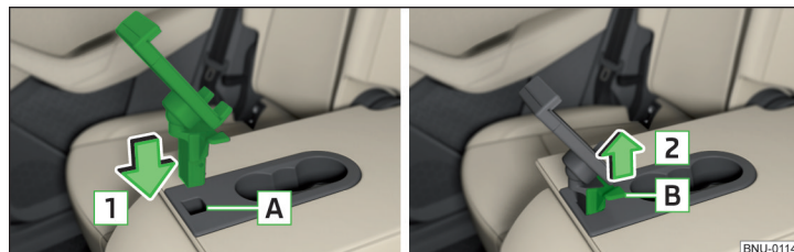
Fig. 134 Installer le support / retirer le support
