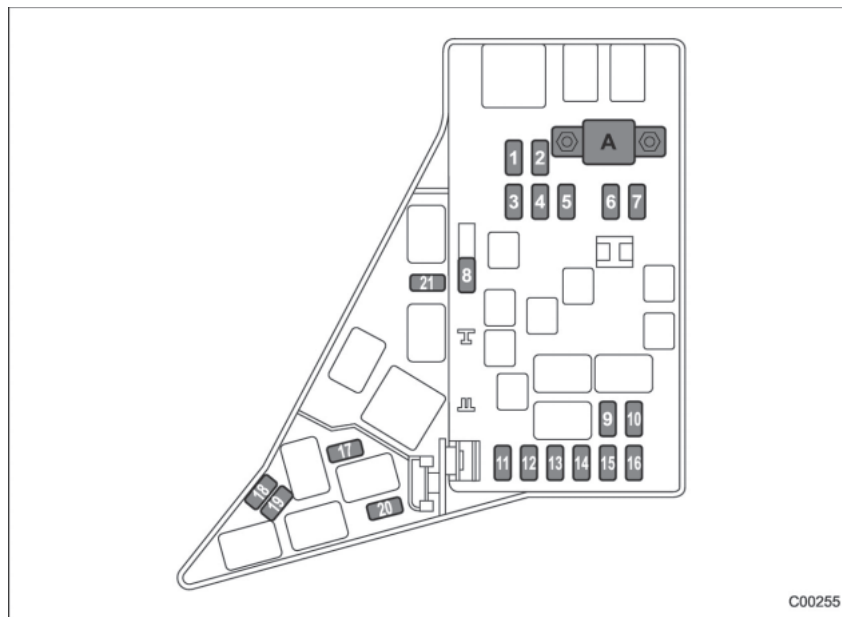
A) Fusible principal
